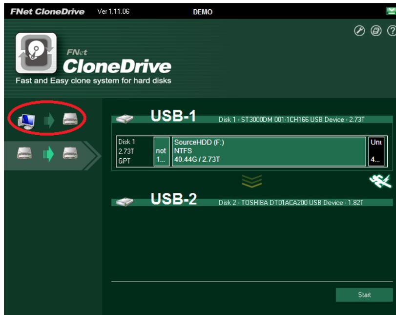
j. Just click the “Start” on the right-down side of the program. Or just push the button on the docking station twice to start the operation.
