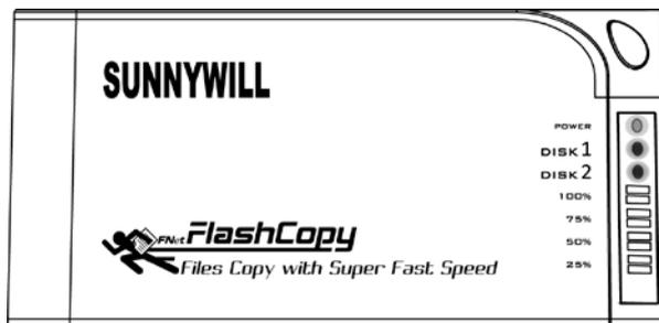
c、 Press and hold the clone button for 3 seconds until the indicator light is blinking, press the button once more for Clone confirmation **while all LEDs are still blinking blue**. Offline clone is starting to process and 25% light will start blinking alone to show its progress.
