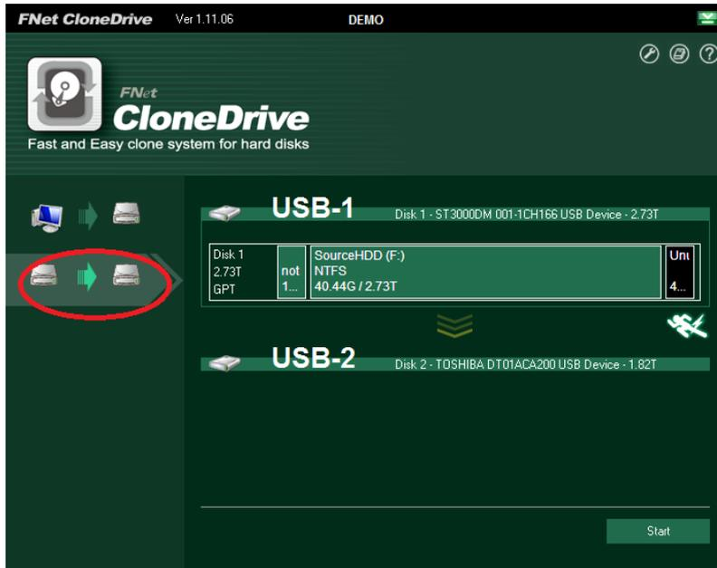
i. User can choose to “Clone system disk to external disk”, which means the system disk inside the PC would be the source HDD, and all the HDD in bay 1, 2 will be the target HDD.
