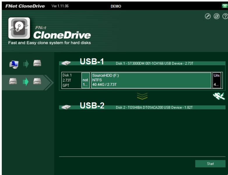
h、 User can choose to “clone the external Disk”, which means the HDD in bay 1 will be the source HDD, and HDD in bay2 are the target HDD.
