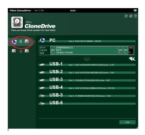
j. Just click the "Start" on the right-down side of the program. Or just push the button on the docking station twice to start the operation.
