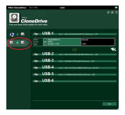
i. User can choose to "Clone system disk to external disk", which means the system disk inside the PC would be the source HDD, and all the HDD in bay 1~6 will be the target HDD.
