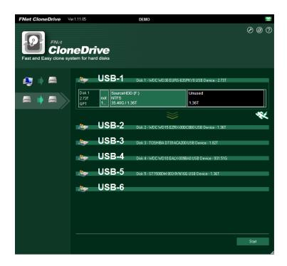
h. User can choose to "clone the external Disk", which means the HDD in bay 1 will be the source HDD, and all the HDD in other bay are the target HDD.
